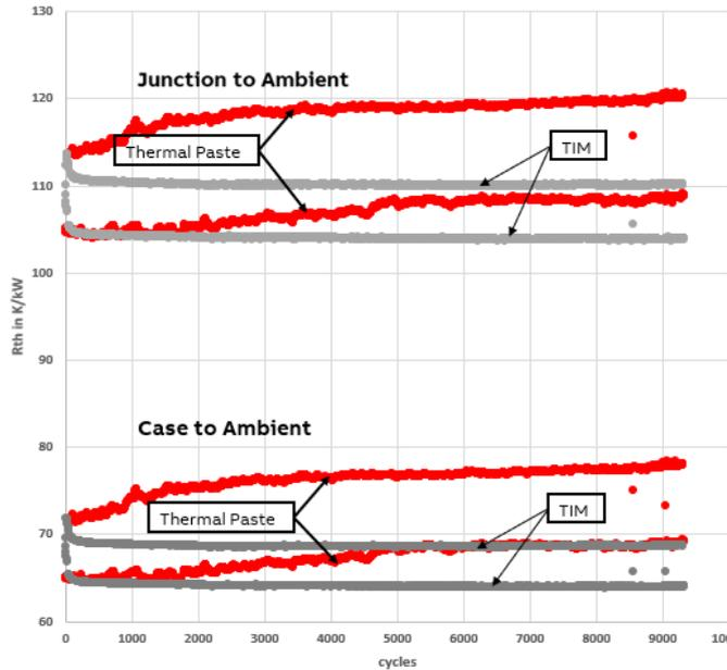
Figure 5: Comparison of TIM and heat conductive paste stability
