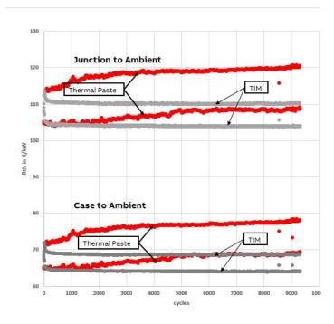
Figure 5: Comparison of TIM and heat conductive paste stability
